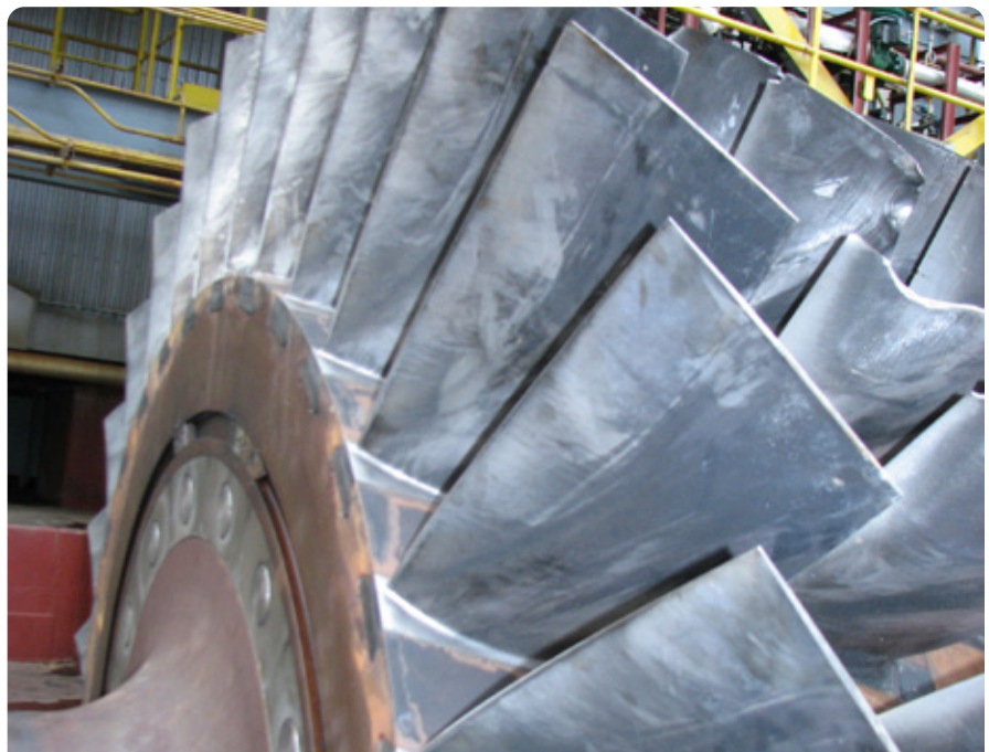
FIGURE 1. Compressor rotor inlet with fouling deposits
