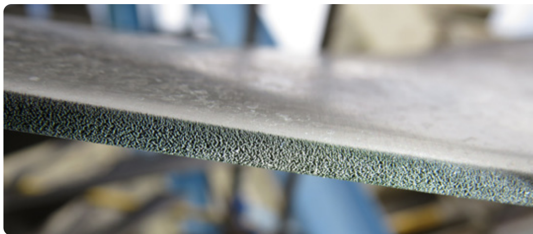
FIGURE 6. Forward compressor blade with leading edge erosion at airfoil mid span
