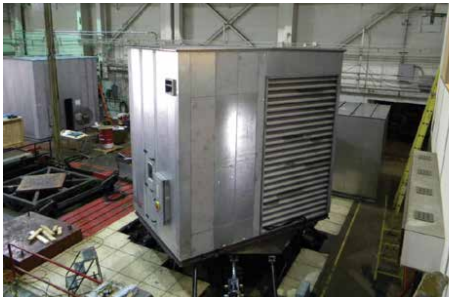
FIGURE 2. Modular air handling unit undergoing seismic testing
