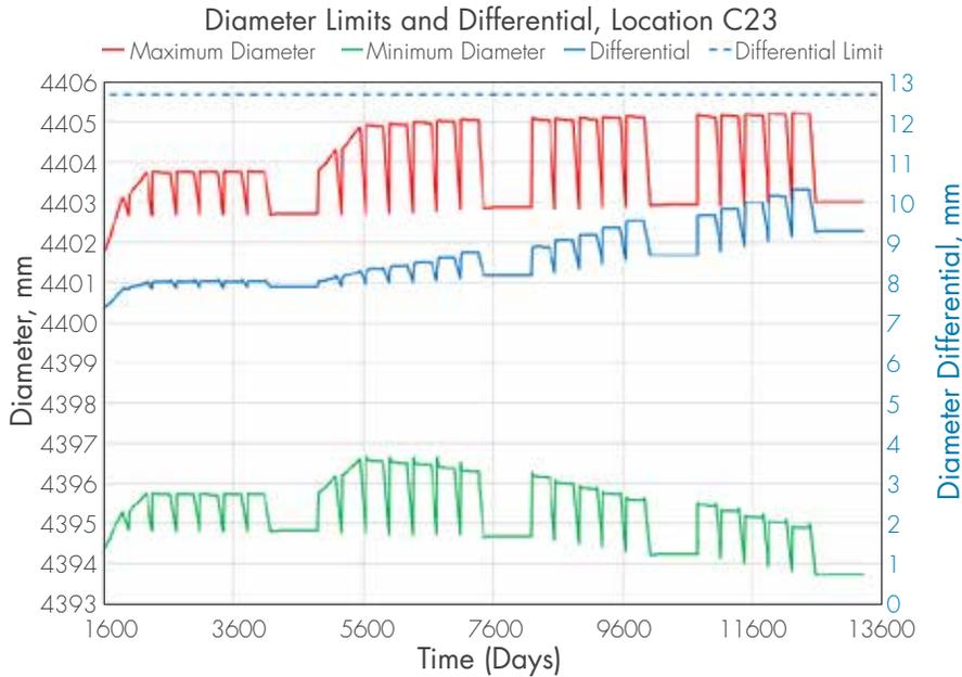
FIGURE 6. Out-of-Roundness Check through Lifecycle, Ratcheting Effect of Power Cycles
