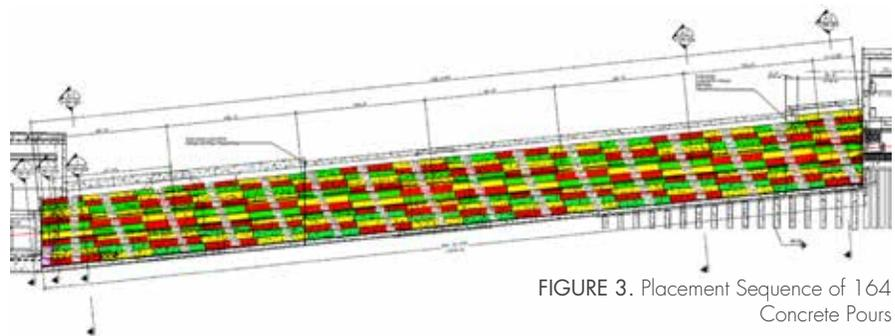
FIGURE 3. Placement Sequence of 164 Concrete Pours
