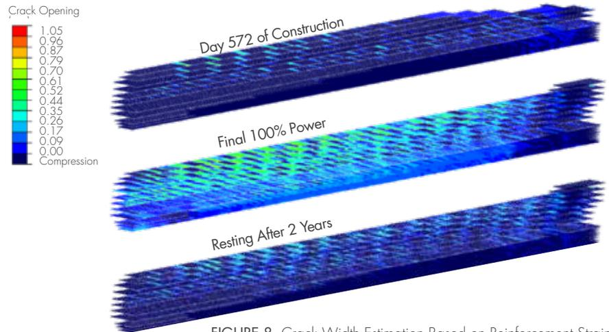
FIGURE 8. Crack Width Estimation Based on Reinforcement Strain
