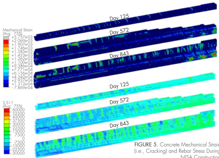
FIGURE 5. Concrete Mechanical Strain (i.e., Cracking) and Rebar Stress During NISA Construction
