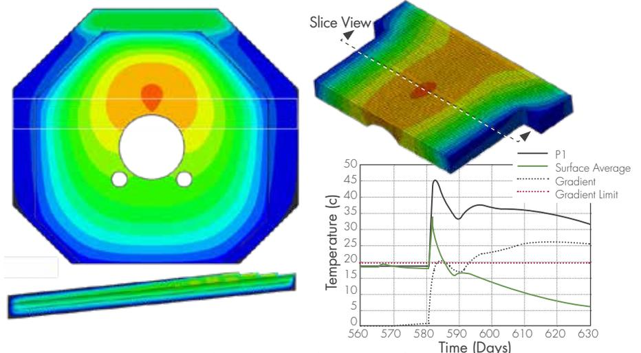
FIGURE 4. Thermal Views and Monitoring of Concrete Placement Temperatures
