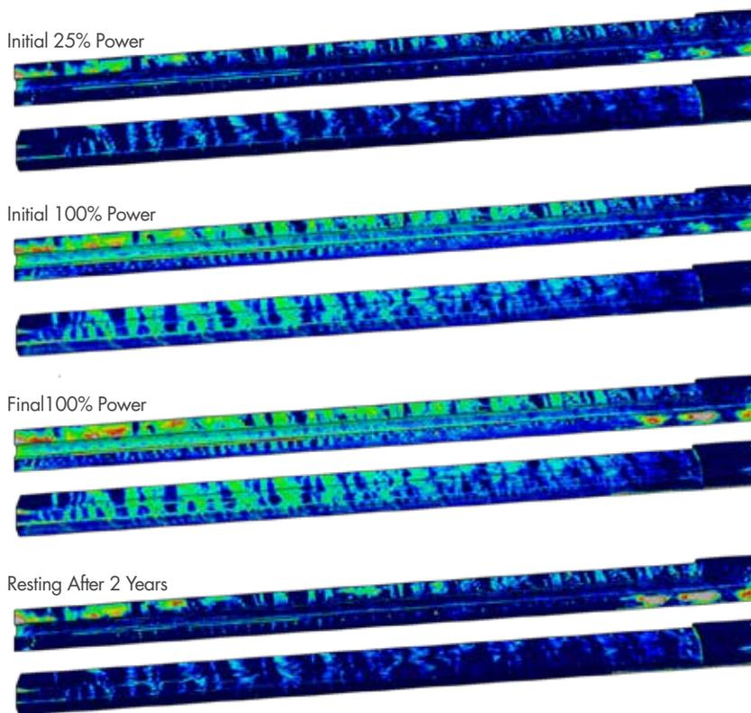
FIGURE 7. Concrete Strains at Various Point in Structures Lifecycle
