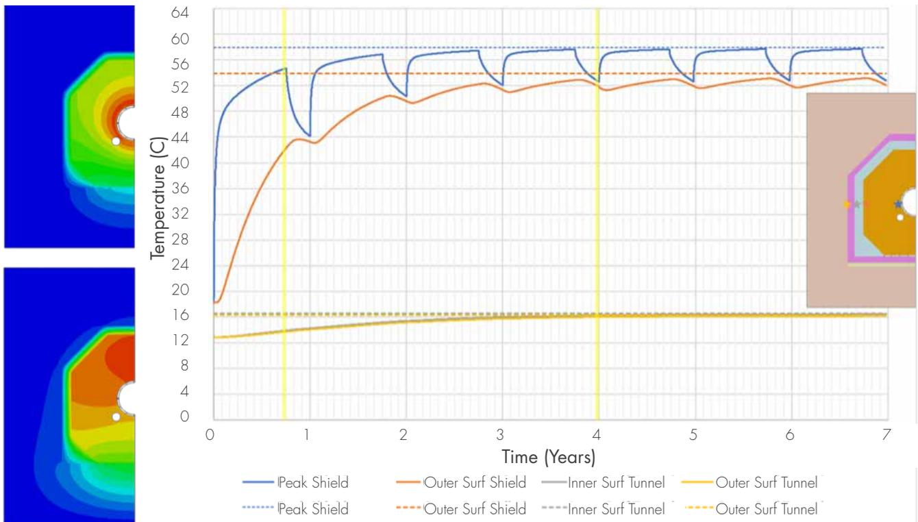
FIGURE 9. 2D Thermal Results of Decay Tunnel, Air Access Space, Shield Tunnel Walls, and Surrounding Soil
