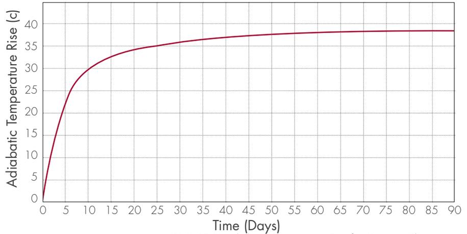
FIGURE 2. Adiabatic Temperature Rise for Concrete Placement
