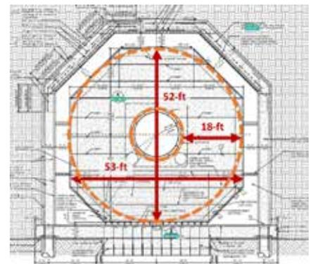
FIGURE 3. Typical Decay Region Tunnel Cross Section
