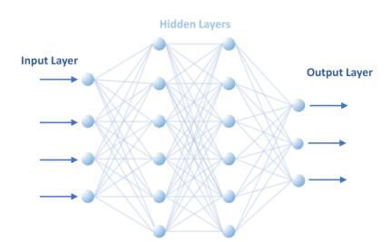
The choice of the number of hidden layers and the number of artificial neurons in each layer are design parameters that are problem dependent and are
